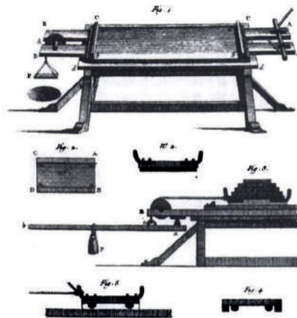
the force of friction that acts on it?'. Coulomb designed simple tests to measure the size of the frictional force when surfaces were sliding across each other at different speeds. He carried out tests and
